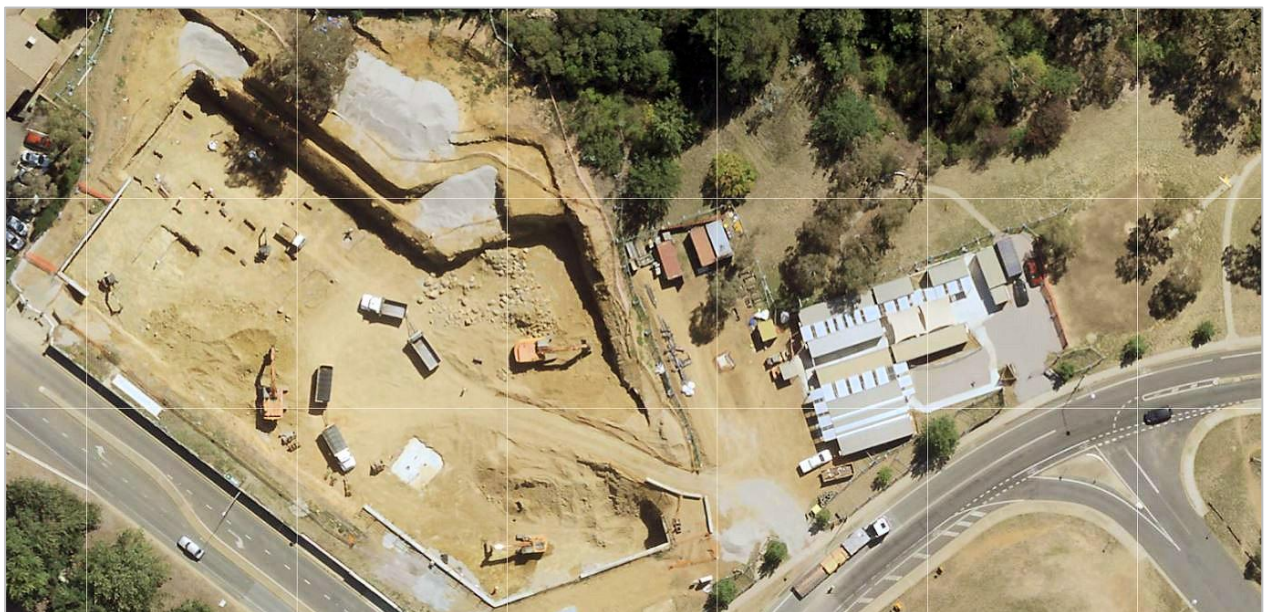
Aerial photograph Mar 2018 [detail] - Excavation of 'Iskia' for foundations and three underground levels, also showing at right works buildings occupying part of the park area (ACTmapi)
