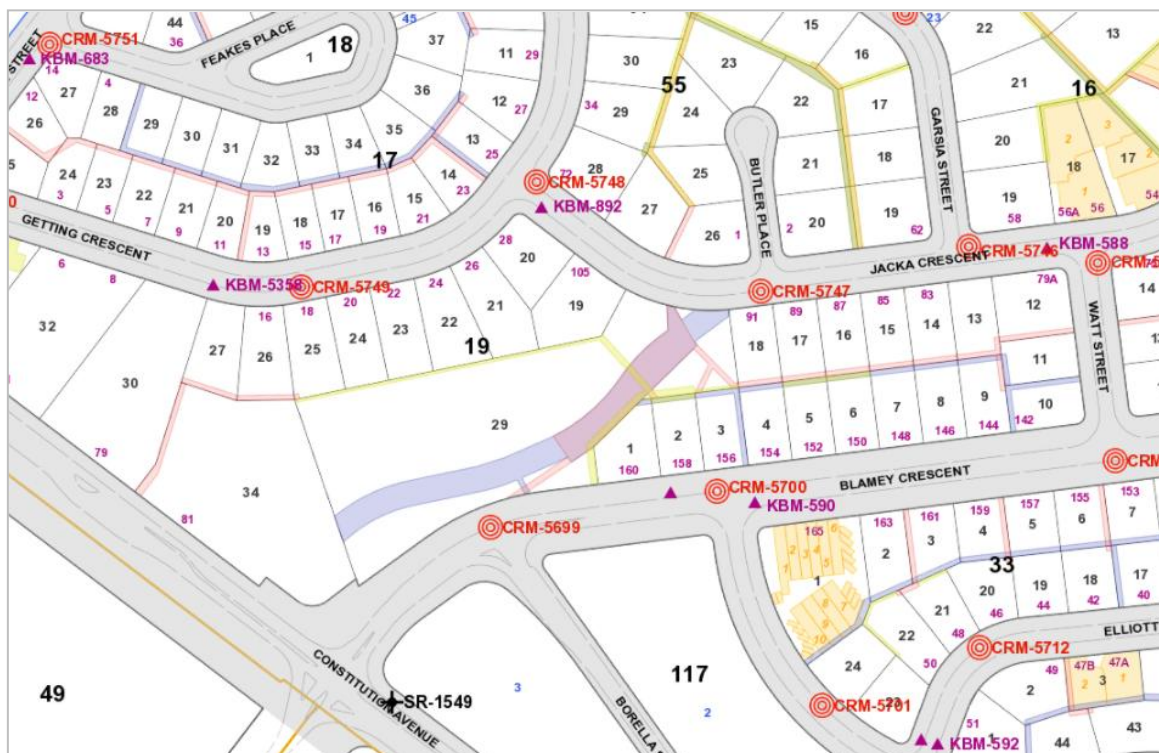
Services infrastructure map [detail] – stormwater and sewer easements shape the park area at centre (Block 29); the mauve shaded stormwater easement has straightened, piped and buried the creek; additional constraints on housing are imposed by the low rocky hill in the upper (northern) half of Block 29 (ACTmapi)
