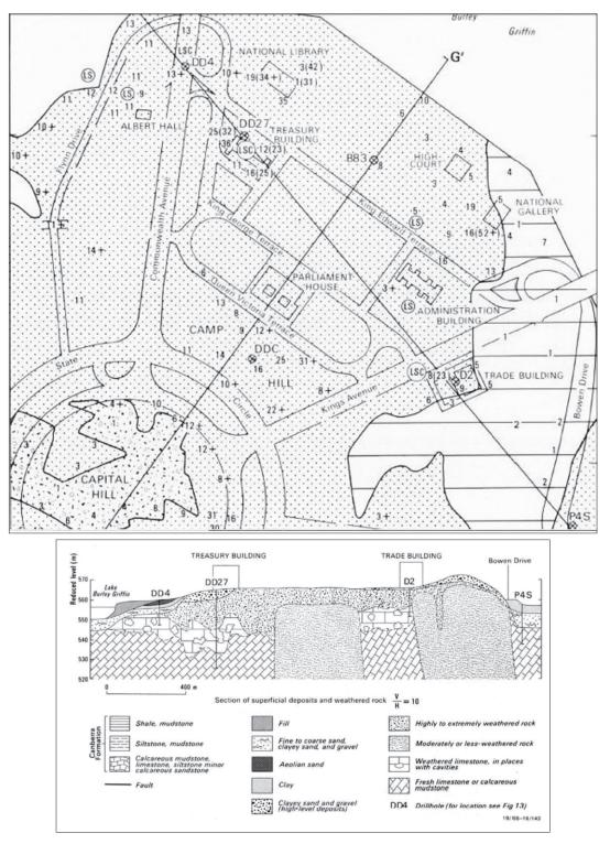
Geological cross-section of the Parliamentary Triangle. The tilted brick pattern is underlying limestone and calcareous mudstone; the punctuated layer above is limestone with cavities.
